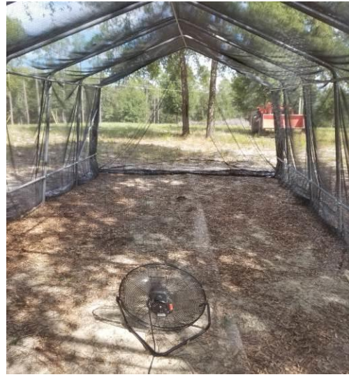
Fig. 5. Fan used to exhaust vapors between tests.
