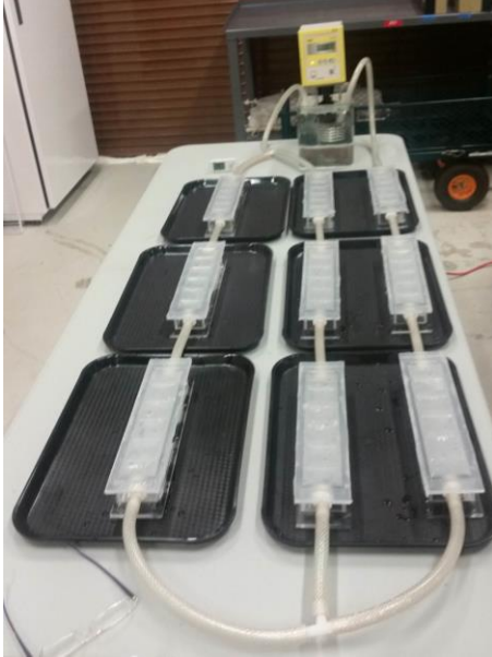
Fig. 6. Lower bases containing surface wells filled with blood substitute covered with collagen and interconnected to temperature-controlled water bath.
