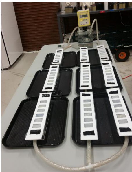
Fig. 5. Treated cloth strips attached to plastic templates placed on top of lower Plexiglas bases.
