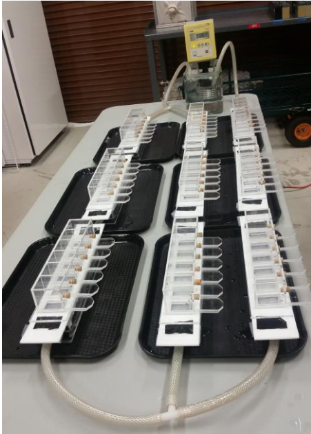
Fig. 1. Upper K&D modules stacked on lower bases and treated cloth-covered templates. Doors opened to expose mosquitoes to treatment surfaces.
