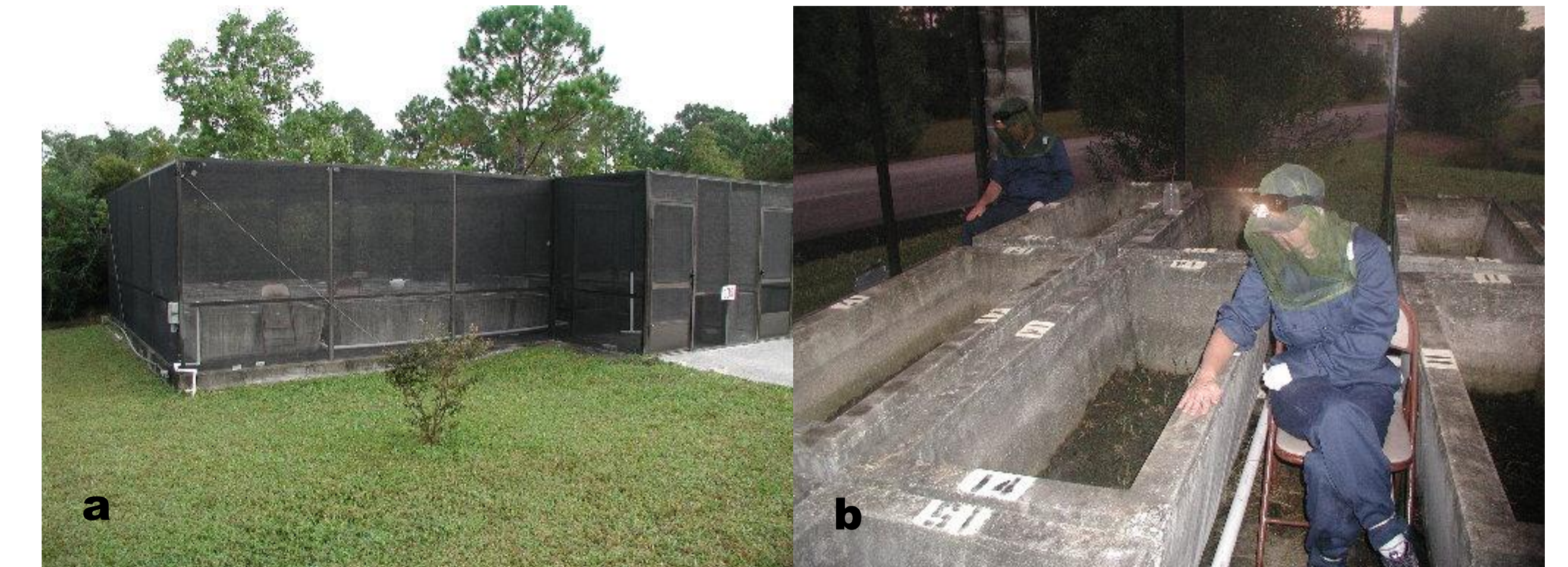
Fig. 3. (a) Area repellent testing enclosure; (b) taking 5-min. biting counts
