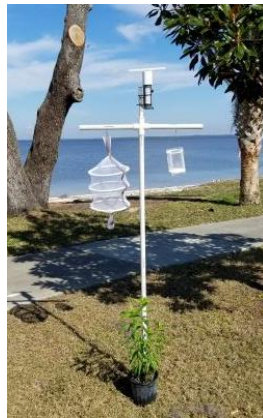
Fig. 5. PVC bioassay and insecticide droplet collection hangers. Milkweed plants at the time of spray test grew to the base of butterfly net.
