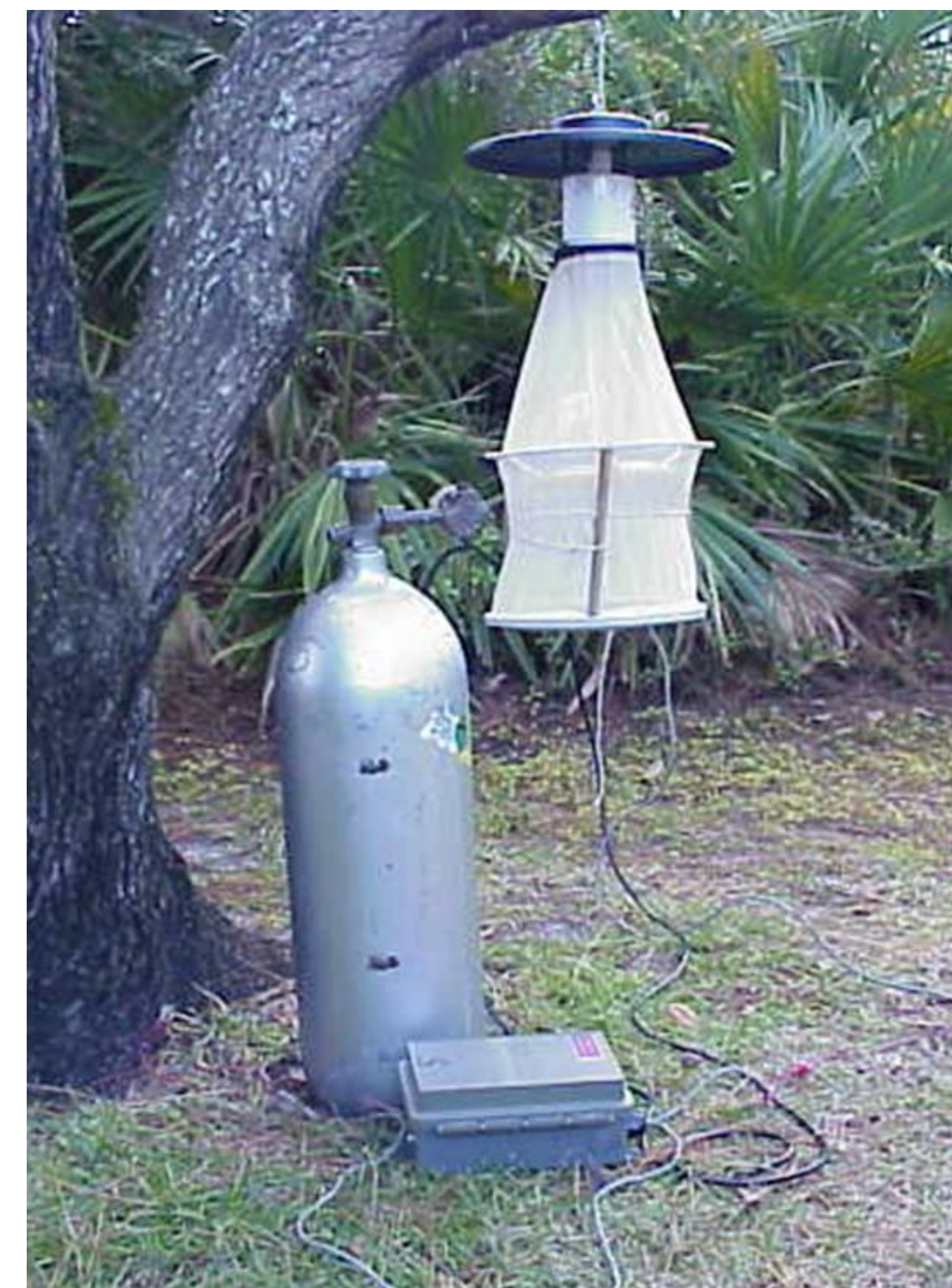
Fig. 2. ABC Light Traps for population monitoring.
